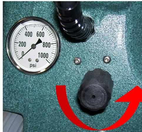
To decrease the solution pressure, turn the regulator knob counter-clockwise.
